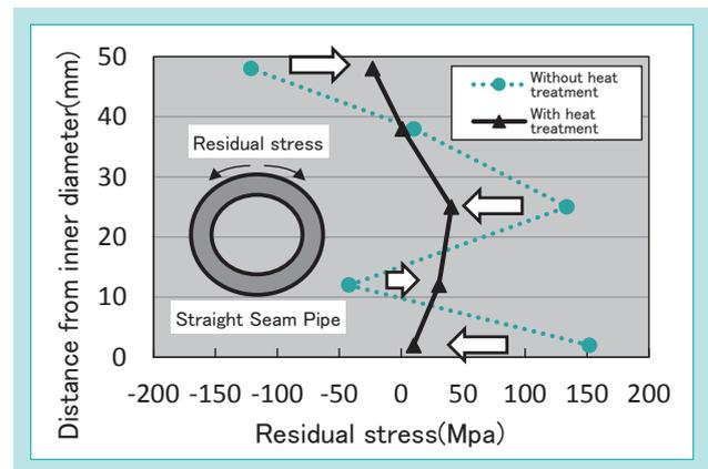
Fig. 7 Stress Relief by Annealing
