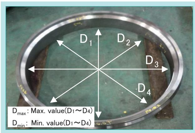
Fig. 6 Measurement Position of Roundness
