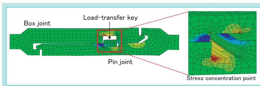
Fig. 8 Stress Concentration Zone of a Mechanical Joint
