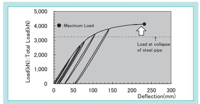
Fig. 11 Four Point Bending Test of Mechanical Joint(2)
