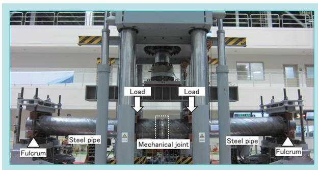
Fig. 10 Four Point Bending Test of Mechanical Joint(1)
