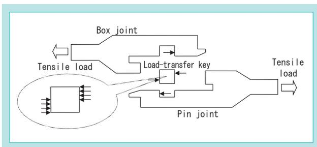
Fig. 4 Force Transfer Mechanism of a Mechanical Joint
