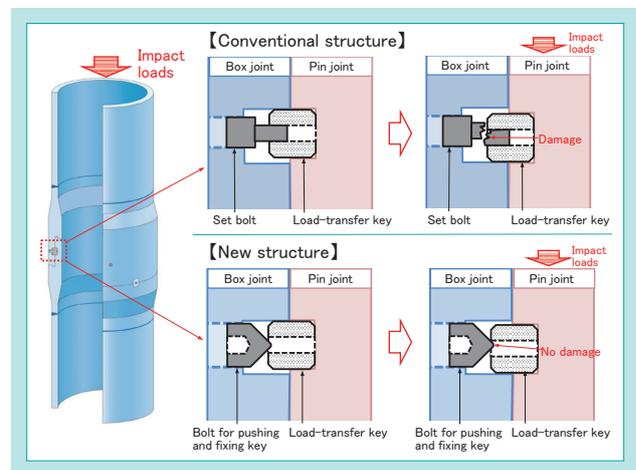
Fig. 14 Improvement of the Fixing Method
