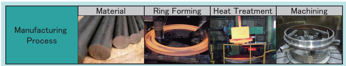
Fig. 2 Manufacturing Process of a Mechanical Joint
