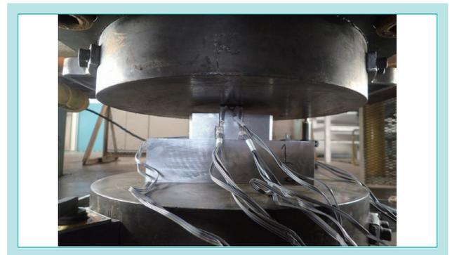
Fig. 9 Bearing Pressure Test of the Load Transfer Key
