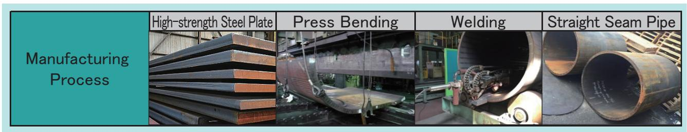
Fig. 3 Manufacturing Process of a Straight Seam Pipe
