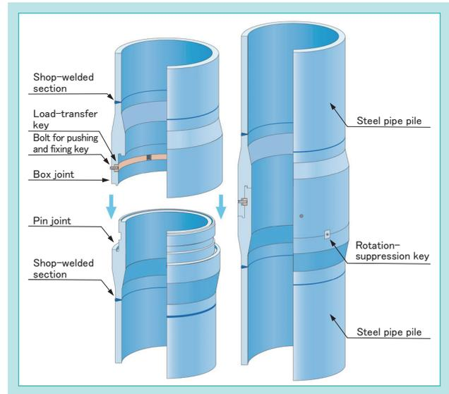
Fig. 1 Mechanical Joint (Laqnican Joint)
